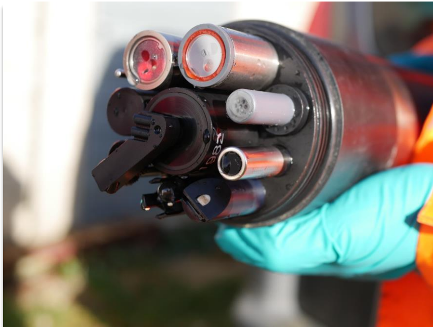
Figure 5-1 Proteus Instruments multi-parameter probe with the protective cage removed
