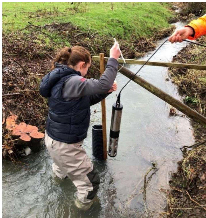
Figure 1: Earthwatch Europe installing a sonde to collect autonomous measurements of water quality. Sondes are placed in stilling wells and regularly monitored.
